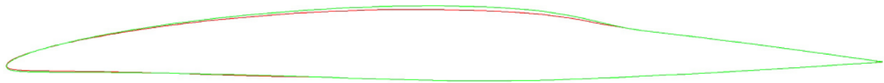
Figure 8. Comparison of the original and DR1 glove using the center span section (original shown in green; DR1 shown in red).
