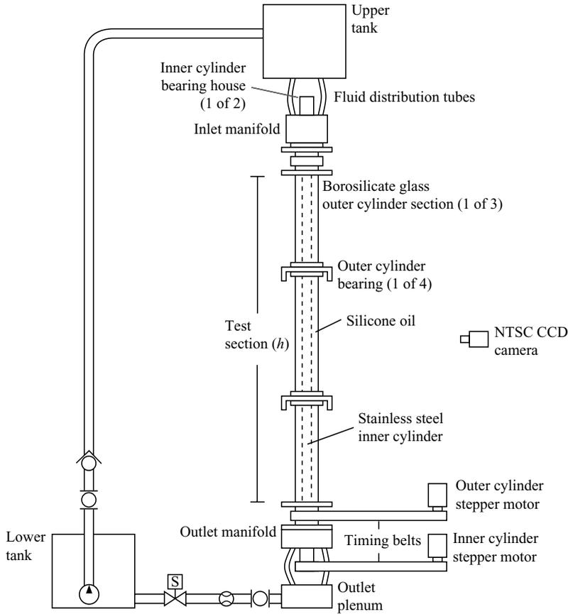
FIGURE 4. Schematic of the experimental apparatus. Overall height is approximately 4.5 m.
